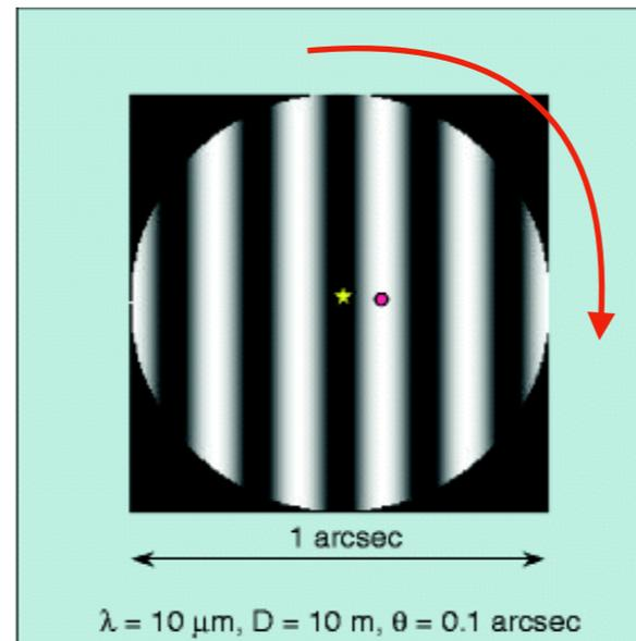
Rotation of the interferometer with the star at the center
