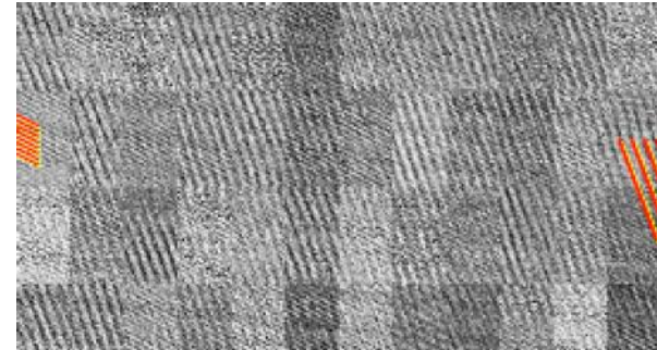
Detector fringes due to electro-magnetic interferences (Li Causi, 2007).
