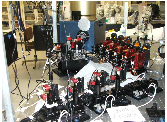
Figure 3: The MIRC combiner at CHARA. The gold-coated off-axis parabolas that focus the incoming telescope beams on the single-mode fibres are visible on the right. At the centre is the PICNIC camera and the focusing optics for the fibred VGroove. Motorised and encoded translation stages are employed everywhere for easy alignment of the optical components of the beam combiner.
