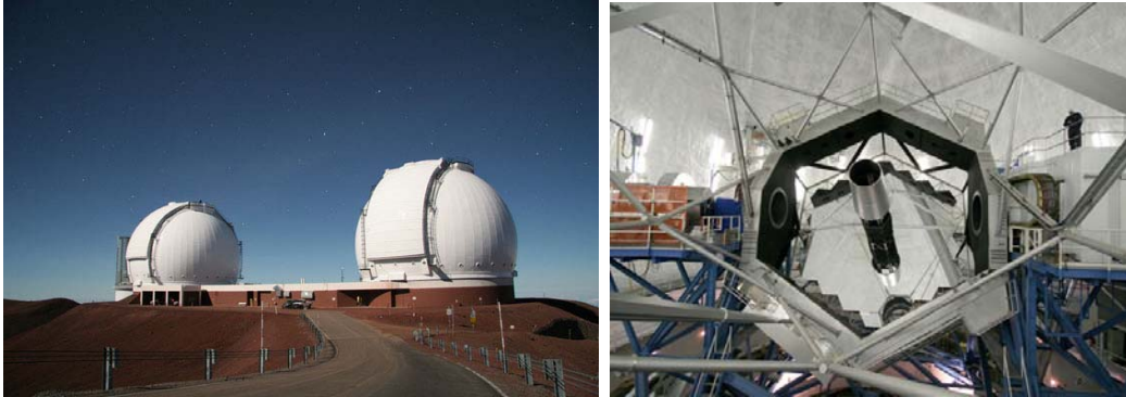
Fig. 1. Left : The domes of the two telescopes of the W. M. Keck Observatory atop Mauna Kea, Hawaii. The telescopes are separated by 85 m and make up the Keck Interferometer. Right : One of the segmented 10 m primary mirrors.
