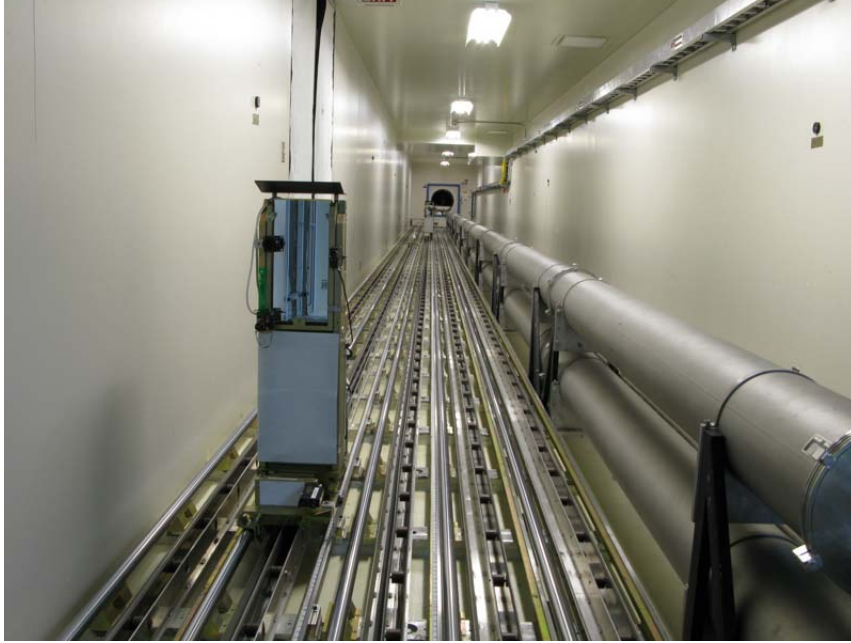
Fig. 4. The quasi-static long delay lines of the Keck Interferometer can correct for \pm 70 m of geometric delay.
