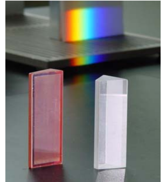
Grism (left) and prism (right) of MIDI
