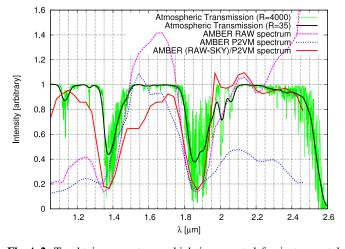
**Fig. A.2.** To obtain a spectrum which is corrected for instrumental effects for the spectral calibration, we subtract from the RAW spectrum the SKY spectrum and then divide by the P2VM spectrum (blue dashed curve). The resulting instrument-corrected spectrum (red curve) is compared with an atmospheric transmission spectrum (green curve: R = 4000; black curve: R = 35).
