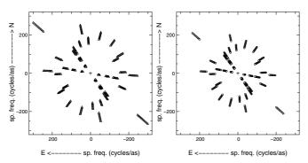
**Fig. 1.** UV coverage obtained on HD87643 in the *H*-band (*left*), in the *K*-band (*right*). The radial lines are caused by the different wavelengths within the bands.
