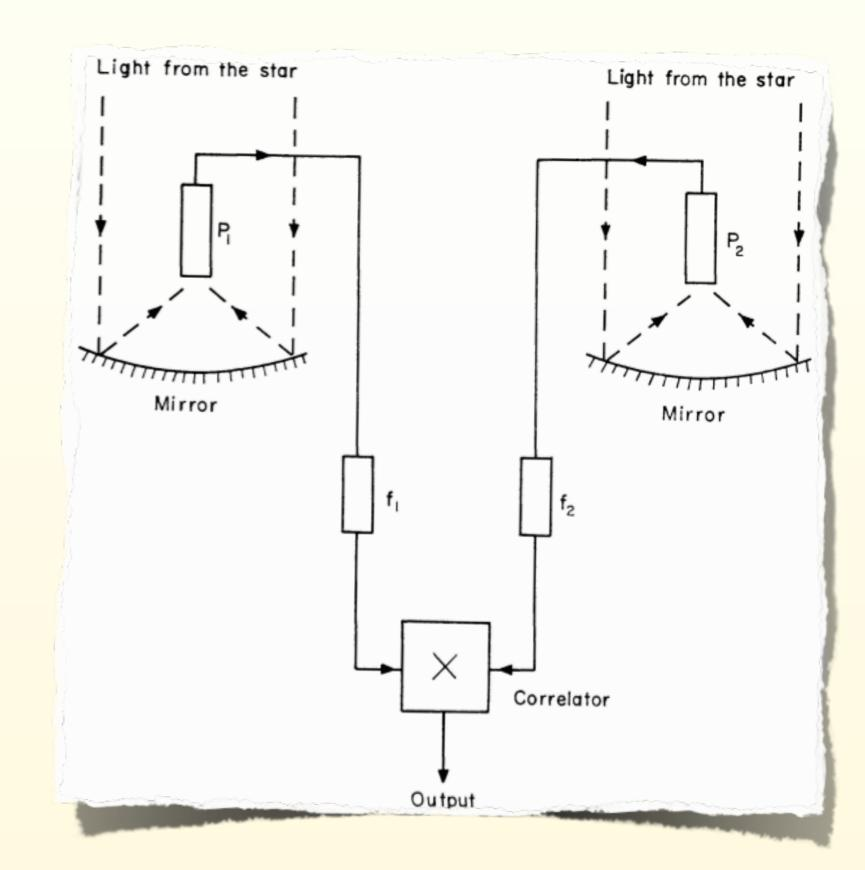
Photomultipliers P1 and P2 count the photons arriving on each of the two apertures
