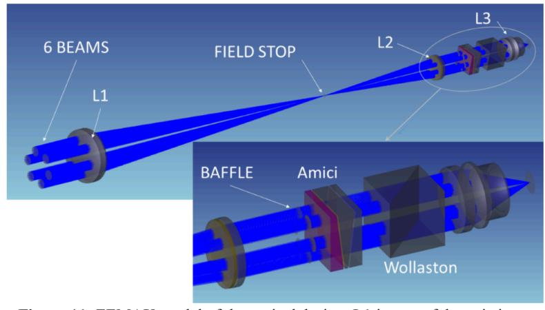
**Figure 11.** ZEMAX model of the optical design. L1 is part of the existing system, while the remaining cold optics are part of this proposal.
