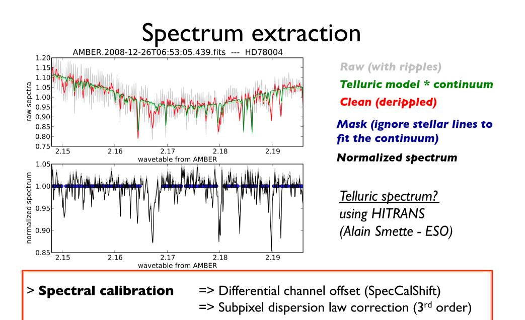
> **Spectrum extraction** => Ripples HR + Continuum fitting + Sky transmission
