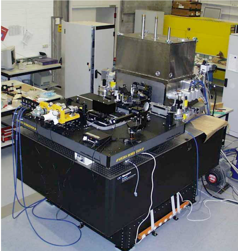
Fig. 4. A view of MIDI in the integration hall at MPIA in Heidelberg. The optics in front are the warm optics. The metallic box in the back is the MIDI dewar.
