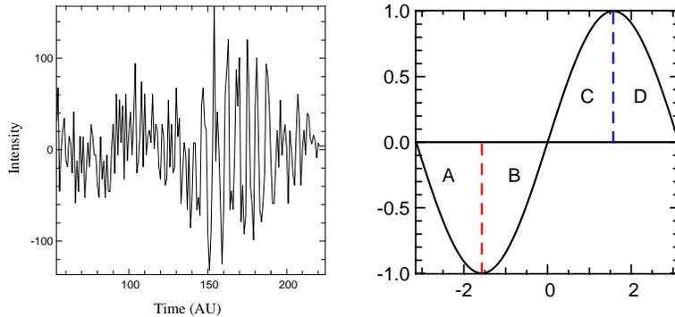
**Fig. 1.** Left: Example of FU Orionis interferogram obtained on Iota. The whole temporal coherence envelope is visible. Right: Sampling of the central fringe at PTI. The raw output of the instrument is a set of four numbers A,B,C and D that correspond to the sample of the flux through four positions in the fringe.
