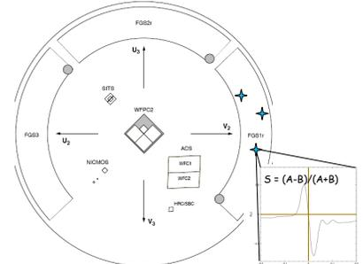
Figure 4: a. (great circle) FGSs in the HST focal plane (projected onto the sky). b. (right panel) FGS1r S-curve response for a point-like source.
