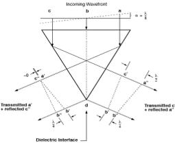
Figure 3: Constructive and destructive interference in the Koester prism.
