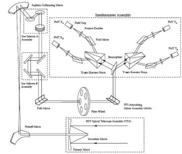
Figure 2: FGS1r optical train schematic.
