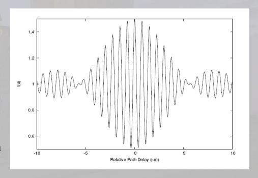
In fact, the fringe amplitude and phase actually measure the amplitude and phase of the Fourier transform of the source brightness distribution at a single spatial frequency.
