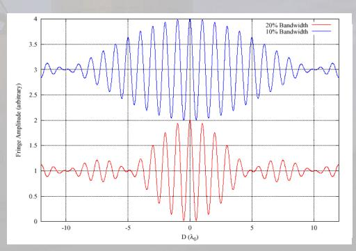
So, the fringes are modulated with an envelope with a characteristic width equal to the coherence length,  $\Lambda_{\rm coh} = \lambda_0^2/\Delta \lambda$ .
