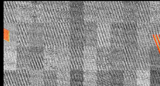
Detector fringes induced by electromagnetic interferences (Li Causi et al. 2007).
