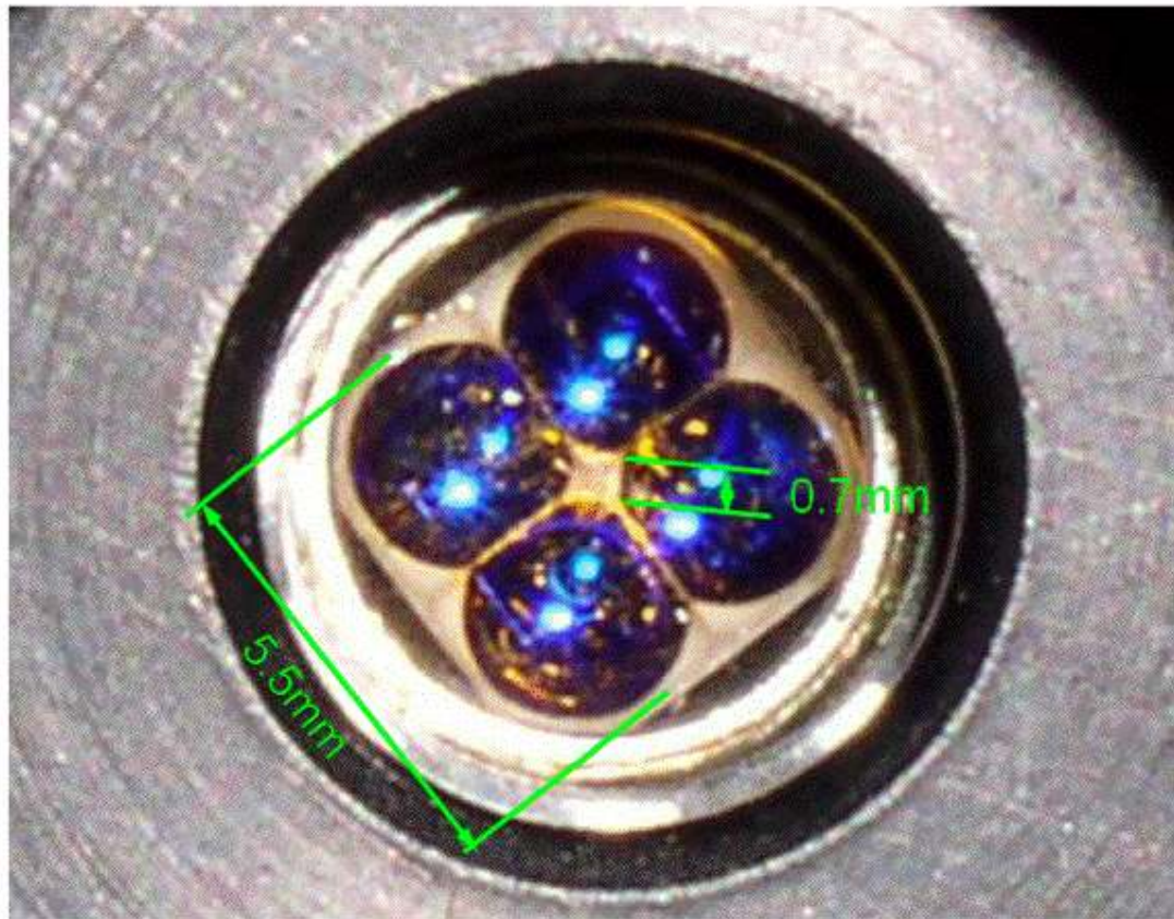
Figure 2: front view of the STRAP head. The 4 lenses are clearly visible. The dimension of the central white square is \sim 0.7\text{mm} . The picture was taken with a digital camera and flash.
