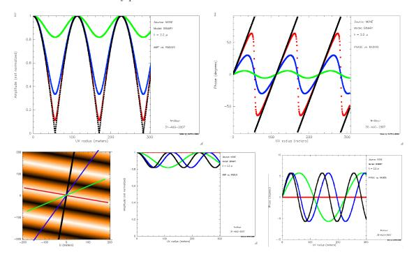
To see how visibility or phase can constrain a binary star model, one just can try to change the baselines orientation and see how visibility and phase vary: this corresponds to the figures at the bottom. You see that the phase is sensitive to the contrast of the binary (top graphs), but also to the position angle (both of the binary star and of the baseline) and of the binary separation. Therefore, the phase can be used instead of the visibility to constrain the binary parameters!
