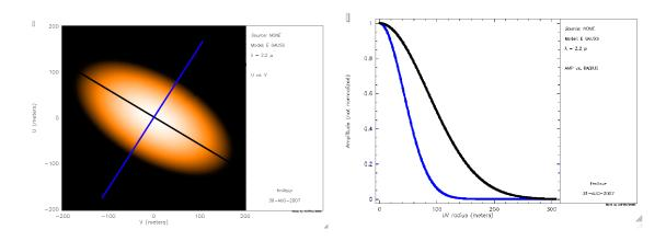
Here is an example of a disk of 2x4 mas (milli-arcseconds) and a position angle of 60 degrees. As one can see, for a given baseline and a varying position angle, the visibility goes up and down, the minimum corresponding to the major axis and the maximum corresponding to the minor axis.
