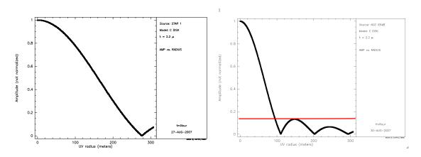
Here, the visibility zeroes around the 280 m baseline. This gives a 1.89 mas diameter for the star, close to the 2 mas input.
