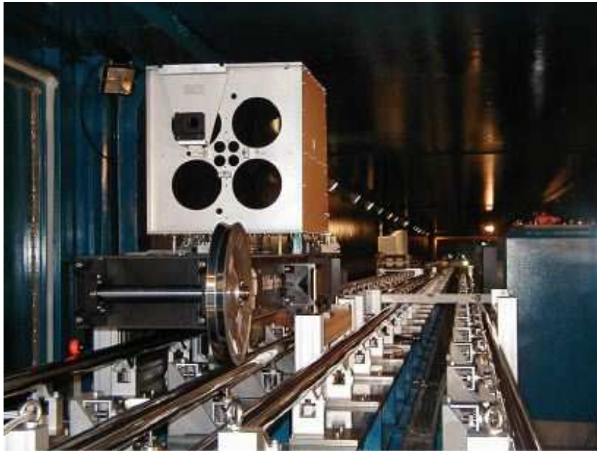
Fig. 3. One of the Delay Lines (with an optical alignment tool inserted in one of the optical paths).
