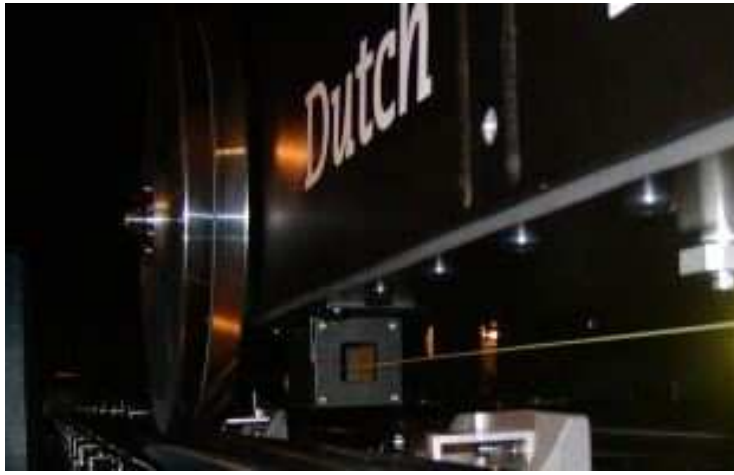
Fig. 9. One capacity sensor and the reference metal wire below a Delay Line.
