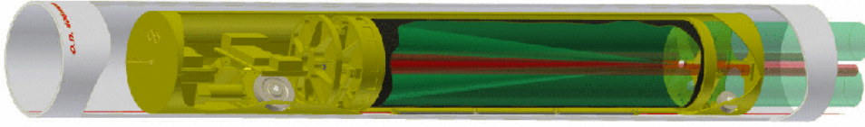
Fig. 2. A schematic cartoon showing of a cat's-eye based delay line. In this design, light enters at the top right, is focused by a parabolic primary onto a flat secondary located at the focus, and reappears to the right as a collimated beam beneath the input collimated beam. The drive wheels for the carriage can be seen at lower right and left, as well as the vacuum vessel in which the whole assembly runs. (Figure courtesy of D. Sun)
