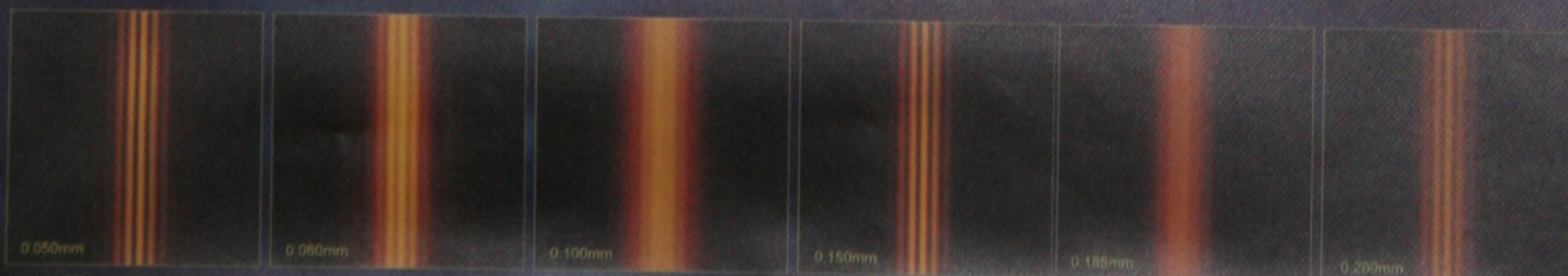
Figure 4. The interference fringes disappear as the slit width increases from 0.050mm (left) to 0.100mm (third from left). The fringes appear again and a second disappearance occurs at 0.185mm.
